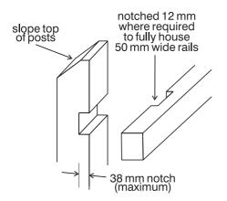
or plinth, palings may project up to 100 mm beyond rails. Rails may be either notched into posts or fixed directly to the face. The maximum depth of notching shall be 38 mm for 100 mm deep posts and 35 mm for 90 mm posts.
